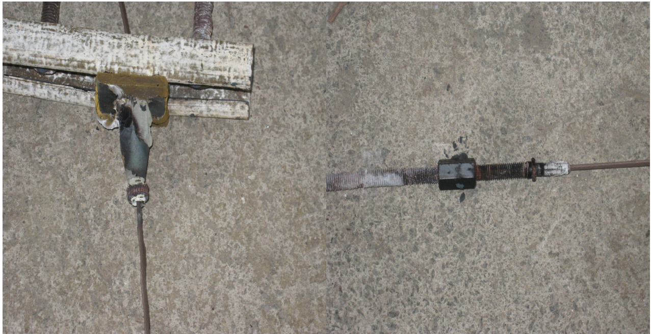
Figure 13 Fixings on removal from the furnace
