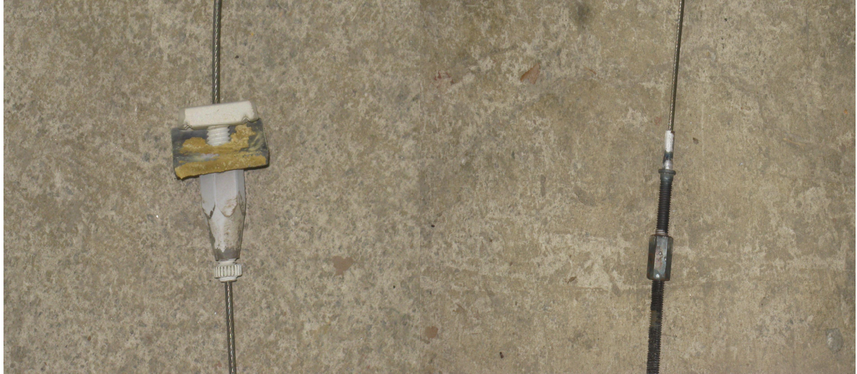
Figure 6 Fixings on removal from the furnace
