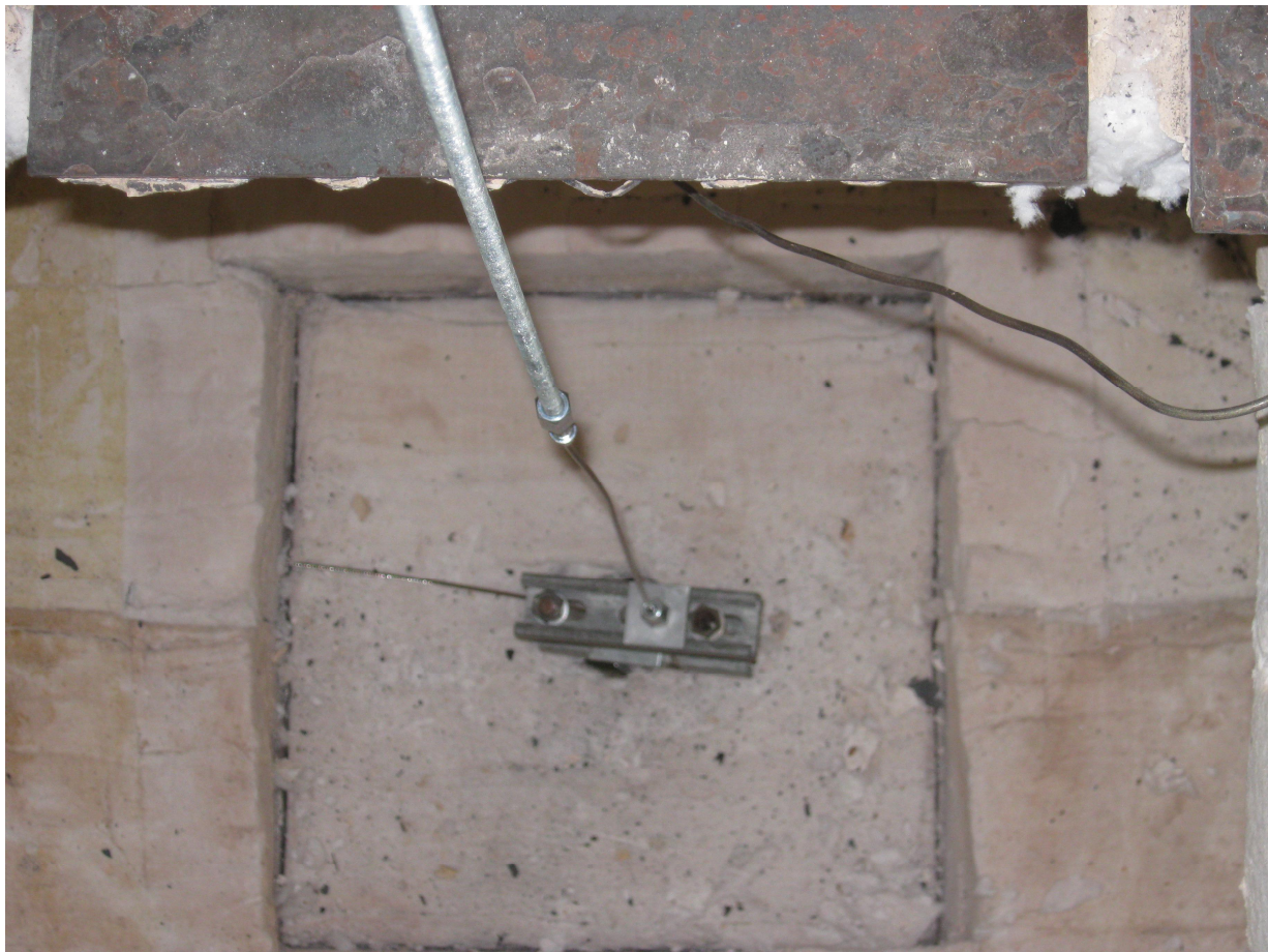
Figure 7 Sample supported on bottom of the furnace at the end of the test
