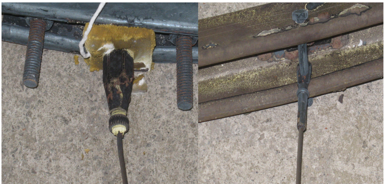
Figure 23 Fixings on removal from the furnace
