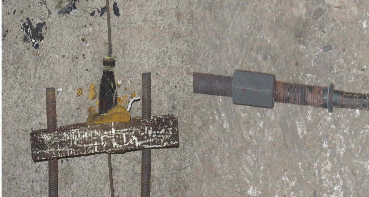
Figure 17 Fixings on removal from the furnace
