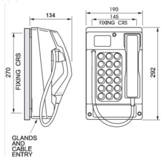
Four 7mm-clearance holes in the Rear Casing (outside the environmental seal) allow it to be screwed or bolted to a wall, or to a pole-side mounting kit (part no 100-02-0208-001).
