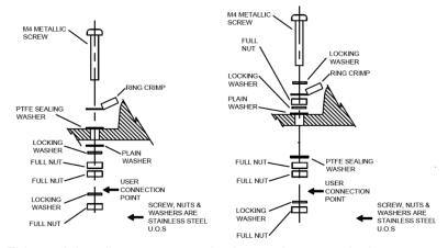
This earth bonding screw can also be used as a continuity connection between glands if 2 metal glands are used.
