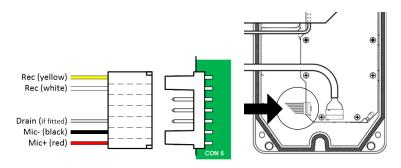
Adapter cables are available for different types of approved headset. Some types have 5 wires (including a drain wire), whilst others have 4 wires (without drain wire).
