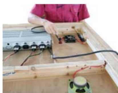
FIG-19 Put down the wires into the sauna cabin
