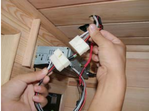
FIG-20 Link the CD connectors
