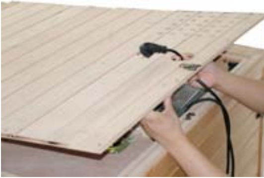
FIG-25 Take out the power plug through external top board
