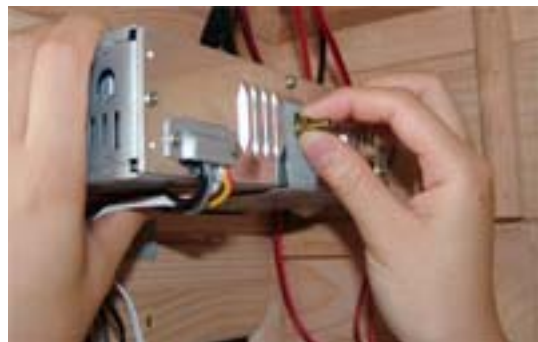
FIG-15.3 Lock the CD with its metal support
