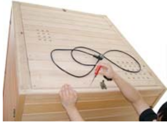
FIG-26 Fix the external board with screw
