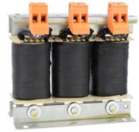
Three phase motor choke VLXM025 25A 0.6mH, suitable for drives size 5.5...11kW
