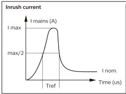
Ecoset 32W 0.4-0.9A 40V I DS W 220-240V 28W System Electrical characte Imax (A) 16 Tref (µs) MCB Luminaires Max. B-10 A 29 B-13 A 38 B-16 A 47 C-10 A 48 C-13 A 63 100% C-16 A 80
