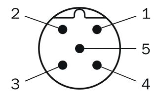
Connector M12, 5-pin, A-coded ① DC 9 V ... 28 V ② "SYNC"/"device ready" ③ GND ④ nc ⑤ nc
