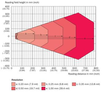
The depth of field is reduced by approx. 10% for devices with plastic lenses.
