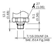
Housing with L-connector (DIN 175301-803 A), IP65
