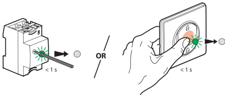
To complete your installation, **briefly** press the **gateway power module** configuration button or **briefly** press the middle of the **wireless master switch**.
