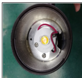
Figure3 Remove the reflector
