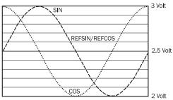
Signal diagram for clockwise rotation of the shaft looking in direction "A" (see dimensional drawing)1 period =  $360^{\circ}$ : 1024 Signal diagram for clockwise rotation of the shaft looking in direction "A" (see dimensional drawing)1 period =  $360^{\circ}$ : 1024
