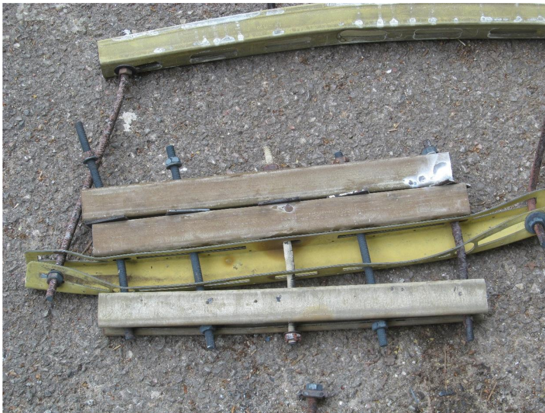
Figure 30 Gripple pipe bracket PB640 following 60 minutes fire exposure
