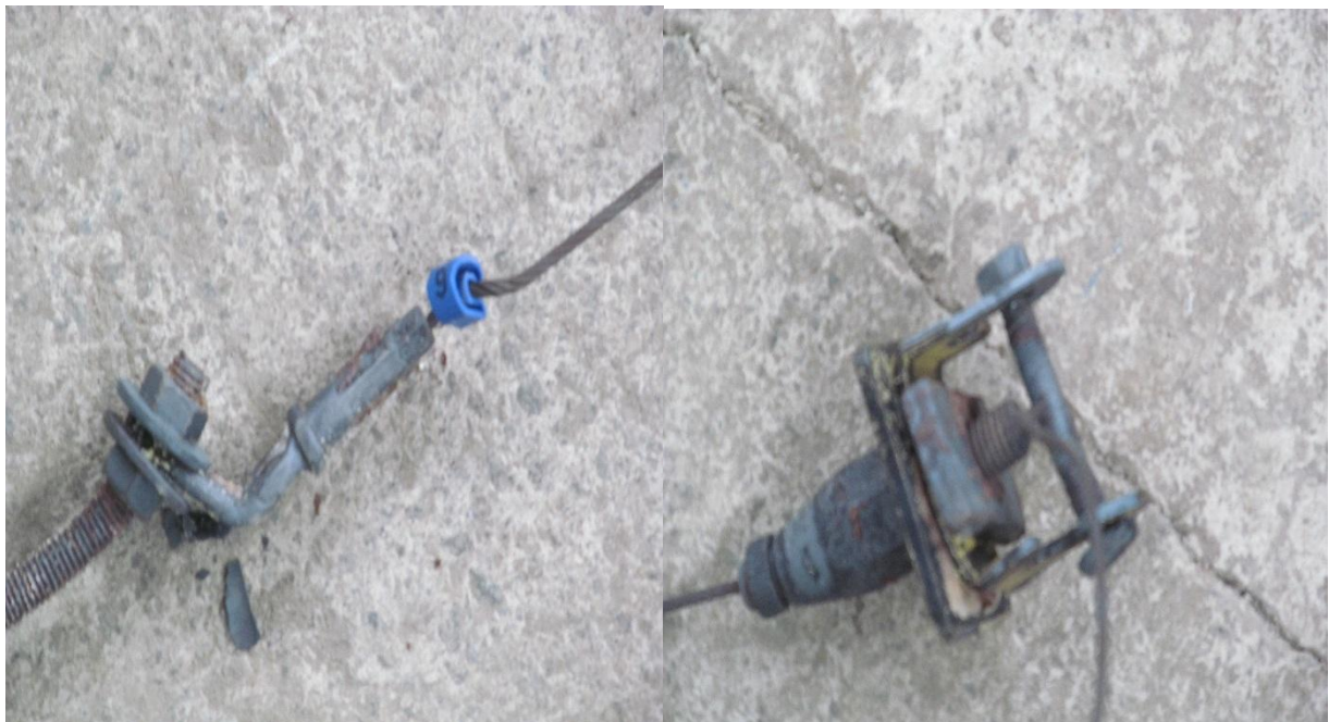
Figure 14 Gripple fixing and 90° eyelet following fire exposure for 120 minutes
