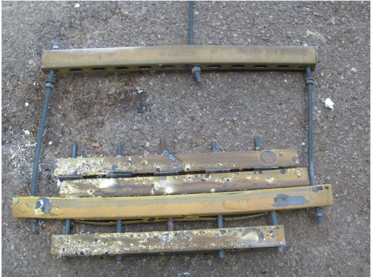
Figure 32 Gripper pipe bracket PB640 following 120 minutes fire exposure
