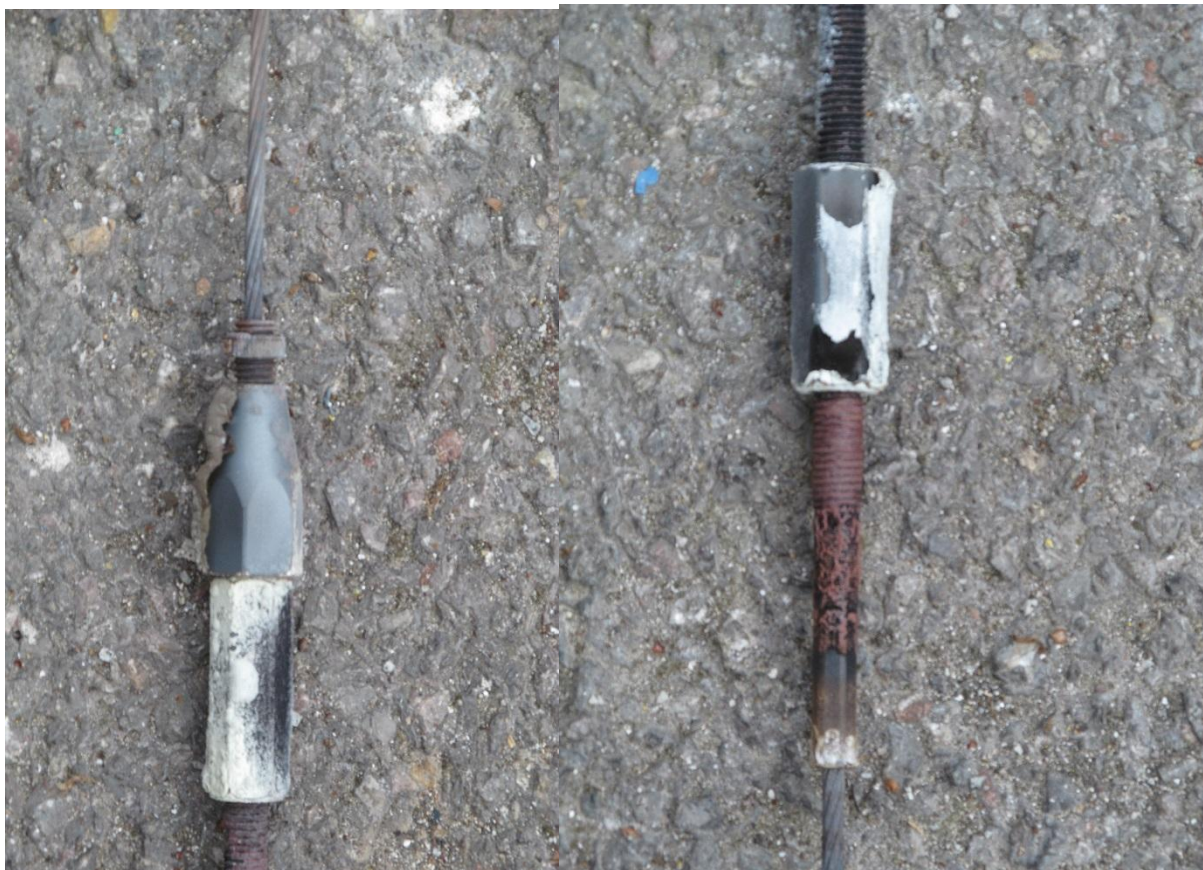
Figure 24 Gripple fixing and M10 stud end fixing following 60 minutes fire exposure
