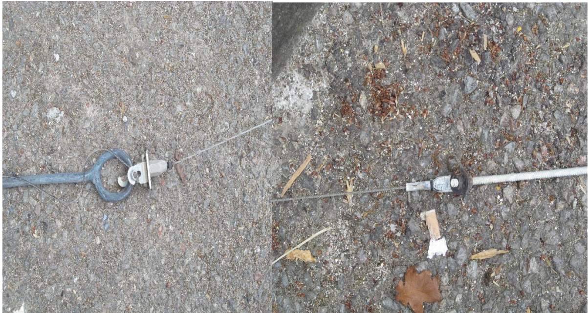
Figure 10 Gripple fixing and 90°eyelet following fire exposure for 30 minutes
