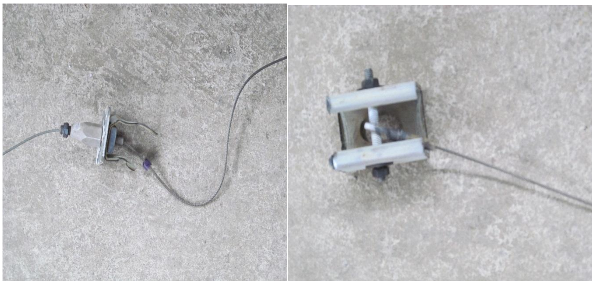
Figure 16 Gripple fixing and straight eyelet following fire exposure for 30 minutes
