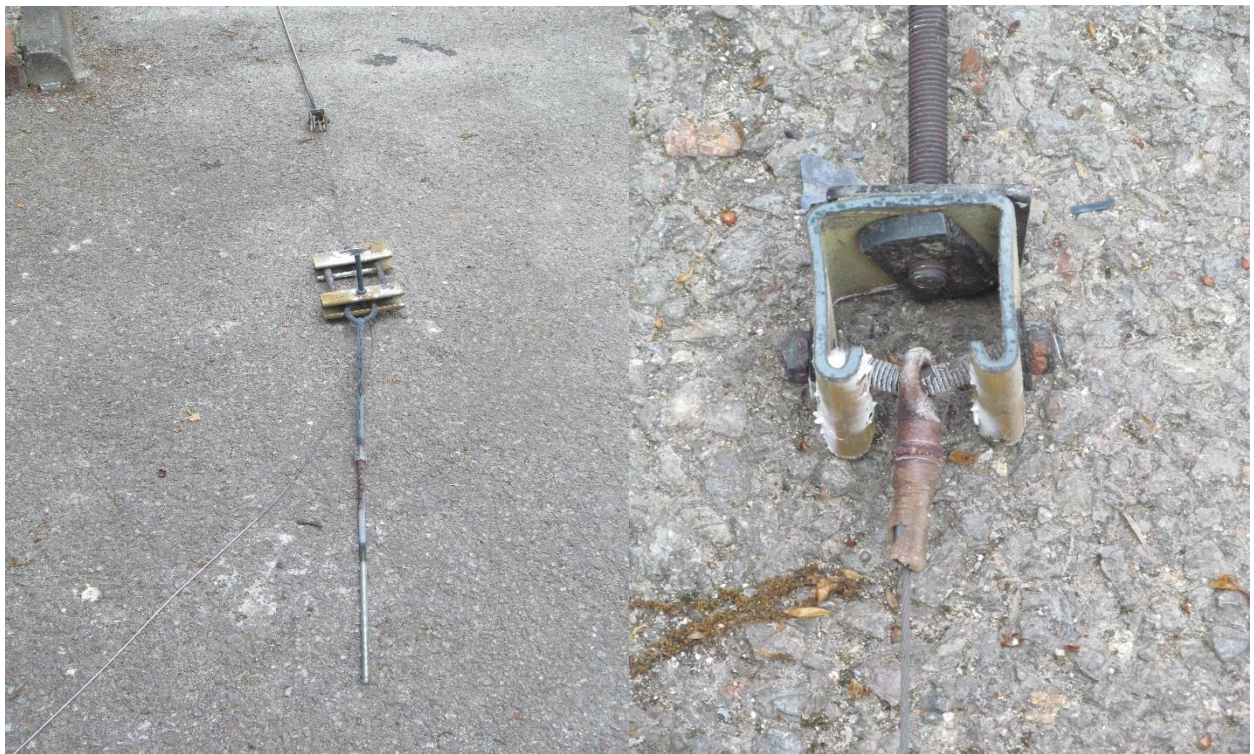
Figure 18 Gripple fixing and straight eyelet following 60 minutes fire exposure
