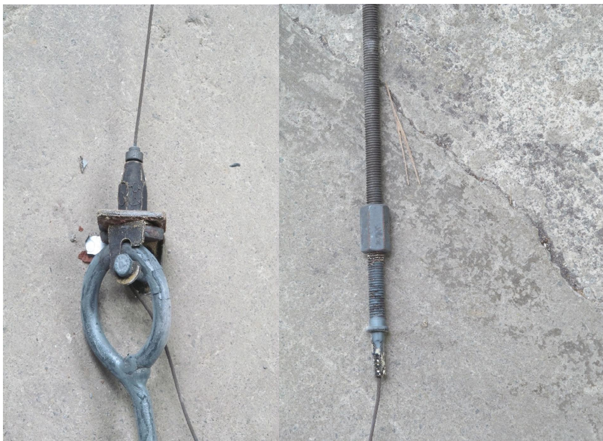
Figure 8 Gripple fixing and threaded connector following fire exposure for 120 minutes
