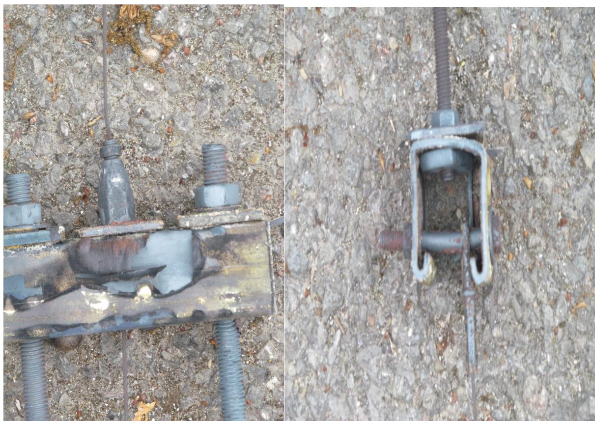
Figure 20 Gripple fixing and straight eyelet following 120 minutes fire exposure
