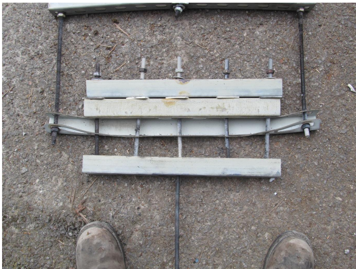
Figure 28 Gripple pipe bracket PB640 following 30 minutes fire exposure
