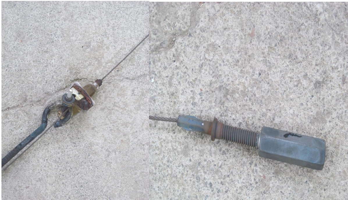
Figure 6 Gripple fixing and threaded connector following fire exposure for 60 minutes
