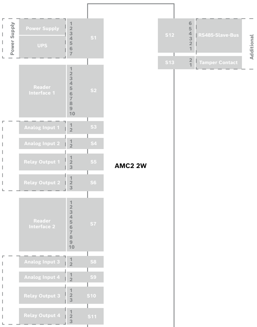
Figure 11.3: Connector blocks of the AMC2-2W
