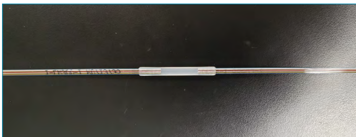
Figure 1: 12-ribbon fiber, post arc procedure.
