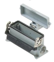
Surface mounting housing, C-TYPE series, with 1 lever, Pg21 x 2 cable entry, size "104.27", with metal cover
