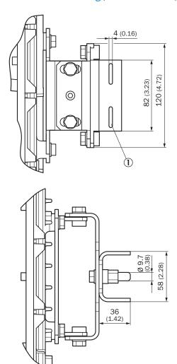
① Groove for tightening straps
