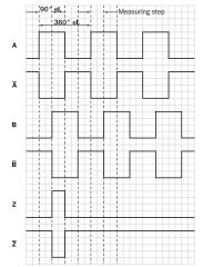
Cw with view on the encoder shaft in direction "A", compare dimensional drawing.
