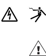
The addition of either symbol to a “Danger” or “Warning” safety label indicates that an electrical hazard exists which will result in personal injury if the instructions are not followed.
