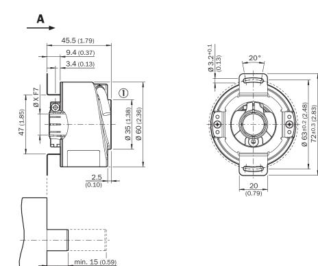
General tolerances according to DIN ISO 2768-mk Cable diameter = 5.6 mm +/- 0.2 mm bend radius = 30 mm
