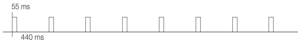
When using several colours, the colour flashes 4 times, being lit for 55 ms and turned off for 440 ms.
