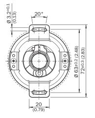
General tolerances according to DIN ISO 2768-mk Cable diameter = 5.6 mm +/- 0.2 mm bend radius = 30 mm
