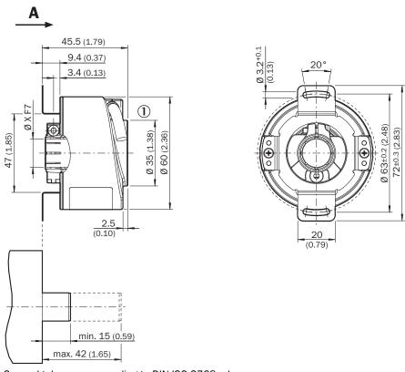
General tolerances according to DIN ISO 2768-mk  $\odot$  Cable diameter = 5.6 mm +/- 0.2 mm bend radius = 30 mm
