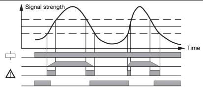
Power supply Object present Signal quality Make switching
