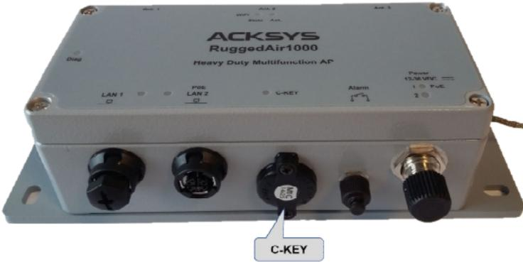
To remove the C- KEY, unscrew the 2 screws of the cover, and then gently pull the device out. If needed, use the screwdriver as a lever, with the help of the notches intended for this purpose at the base of the screw guides.
