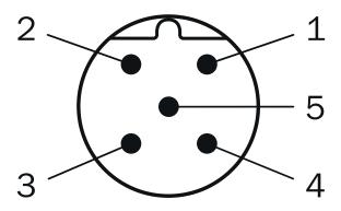
Connector M12, 5-pin, A-coded
