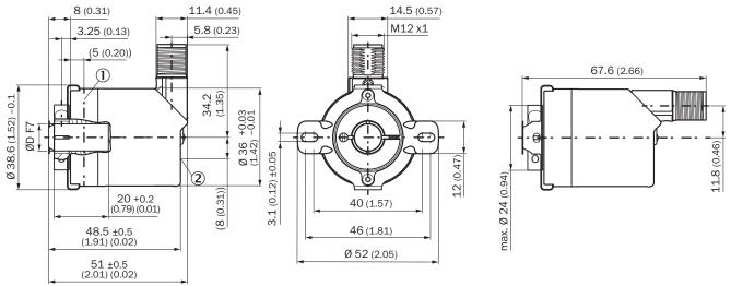
① Measuring point for operating temperature
