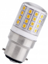
142595 LED B22d T27X58 100V-260V 4W (42W) 500lm 830 Clair
