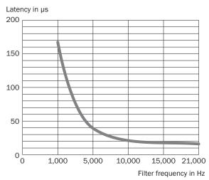
Adjustable filter frequencies 21 kHz, 15 kHz, 10 kHz, 5 kHz und 1 kHz - Default setting 21 kHz Error limits
