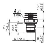
Housing with circular plug-in connector M12 x 1
