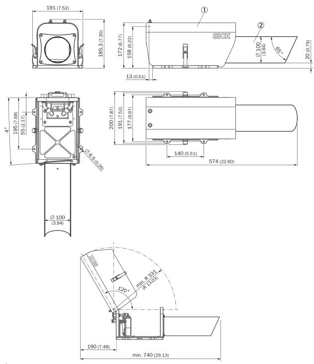
Heavy-duty protective housing with water cooling (part number 2087692)
