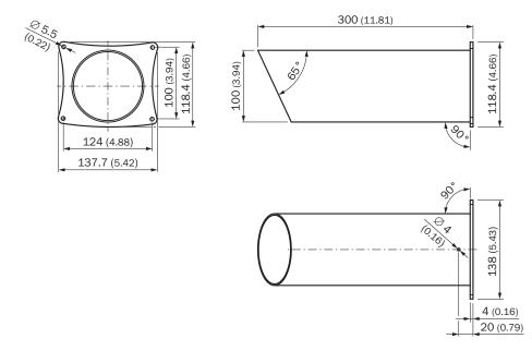
Heavy-duty protective housing with water cooling and tube
