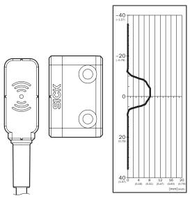
Safe switch on distance  $S_{ao}\,6\;\text{mm}$
