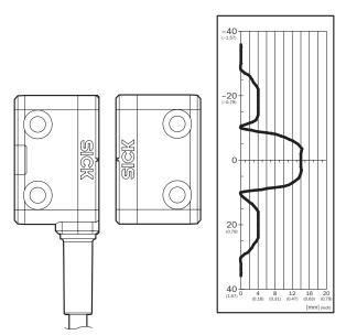
Assured switch on distance Sao 10 mm. Observe border areas for parallel approach: a minimum distance of 6 mm (typical) must be upheld when the actuator moves laterally to the sensor surface. This prevents early triggering due to the side preparation areas.
