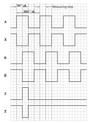
CW with view on the encoder shaft, compare dimensional drawing.Interfaces G, P, R perform only the channels A, B, Z.
