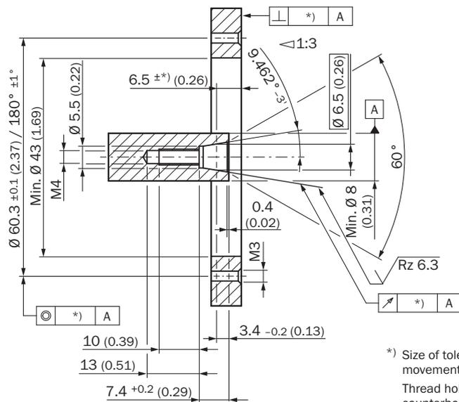
\*) Size of tolerance reduce the allowed movement of the shaft, see data sheet.
