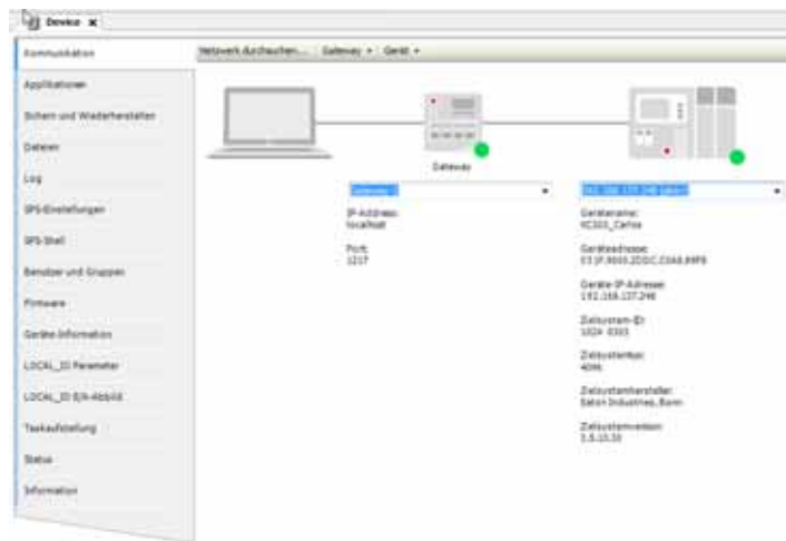
Figure 64: Successful connection between PC and XControl PLC
