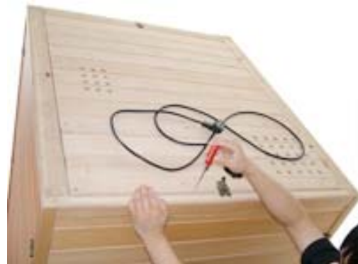
FIG-24 Fix the external board with screws
