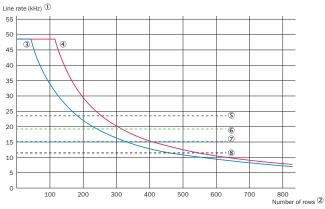
The maximum line rate is based on the number of sensor lines used Line rate (kHz)
