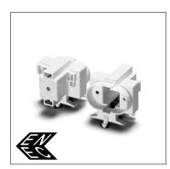
G23 surface-mounted lampholder Casing: PBT GF, white, T140 Nominal rating: 2/250 Push-in twin terminals: 0.5-1 mm<sup>2</sup> Fixing holes for screws M4 Central fixing hole for screw M3
