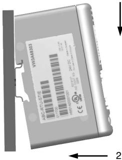
Start by placing the module rear base on the top of the rail, pushing downwards (1) to compress the module spring. Then push the module against the DIN rail (2) until the base of the module casing clips onto the rail.
