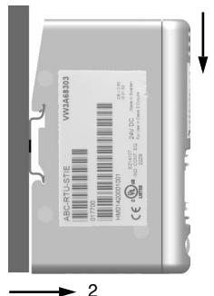
Start by pushing the module downwards (1) to compress the module spring. Then pull the bottom of the module casing forwards (2) until the back of the casing unclips from the rail.
