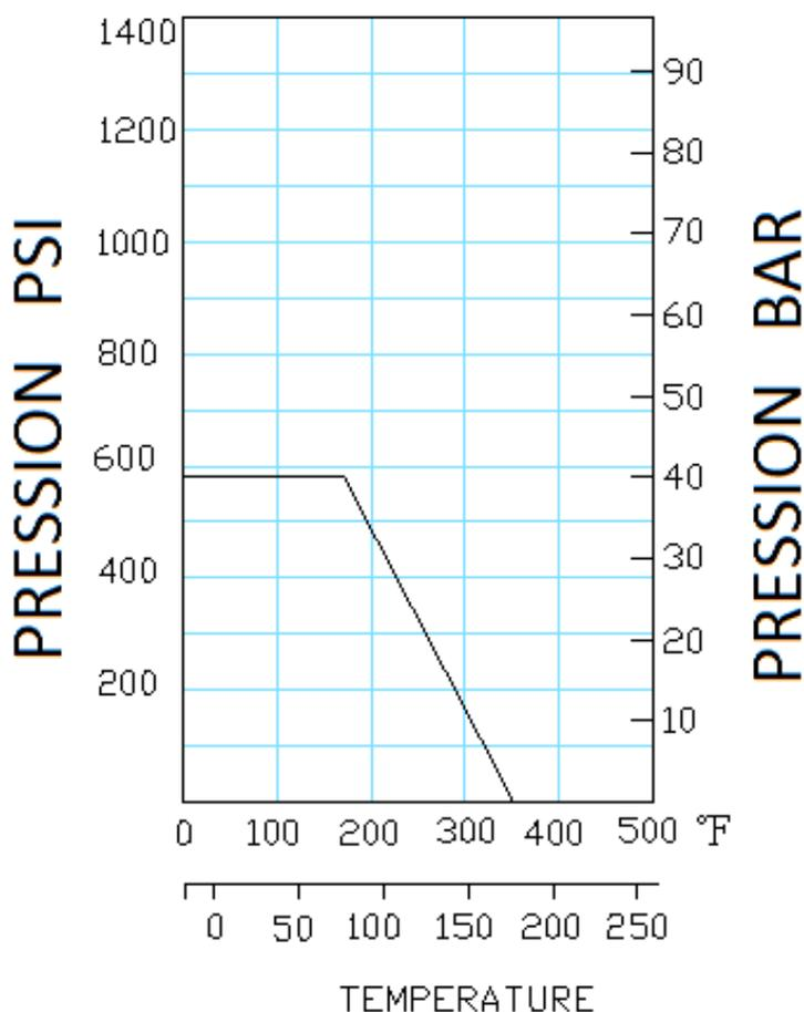
**ROBINET A TOURNANT SPHERIQUE 3 PIECES A BRIDES PN40 ACIER A216WCB DIN 3202-1 F1**
