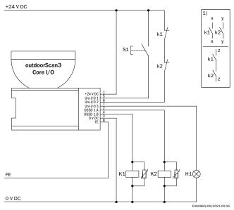
① Output circuits: These contacts must be incorporated into the control such that the dangerous state is brought to an end if the output circuit is open. For categories 4 and 3, they must be incorporated on dual-channels (x, y paths). Single-channel incorporation into the control (z path) is only possible with a single-channel control and taking the risk analysis into account.
