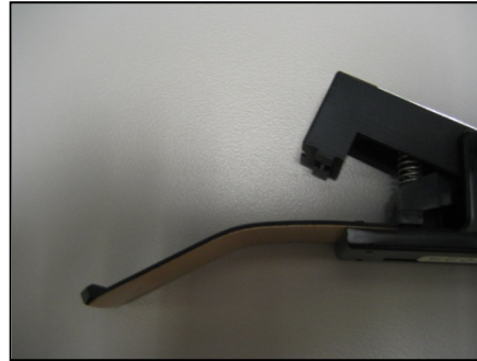
Figure 11 - Damaged Base Plate
