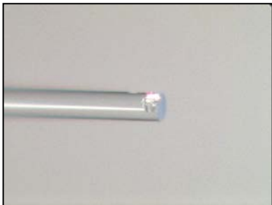
Figure 5 - Bad Cleave (microscope)
