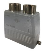
Hood, C-TYPE series, with 2 pegs, Pg21 x 2 top cable entry, size "77.27", high construction
