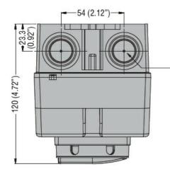
PG13.5 / M20 PG16 / M25 knockouts on top and bottom
