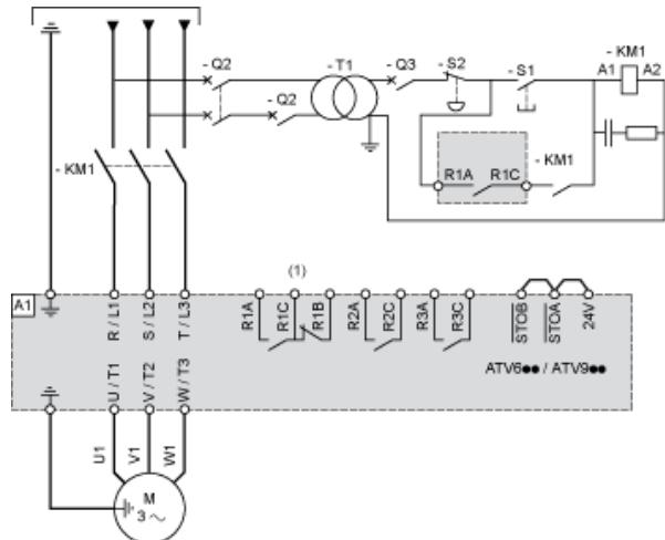
(1) Use digital output R1 set to operating state Fault to switch Off the product once an error is detected.
