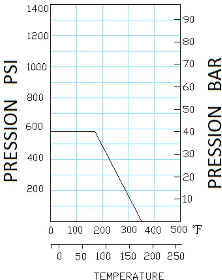
**ROBINET A TOURNANT SPHERIQUE 3 PIECES A BRIDES PN40 INOX CF8M DIN 3202-1 F1**
