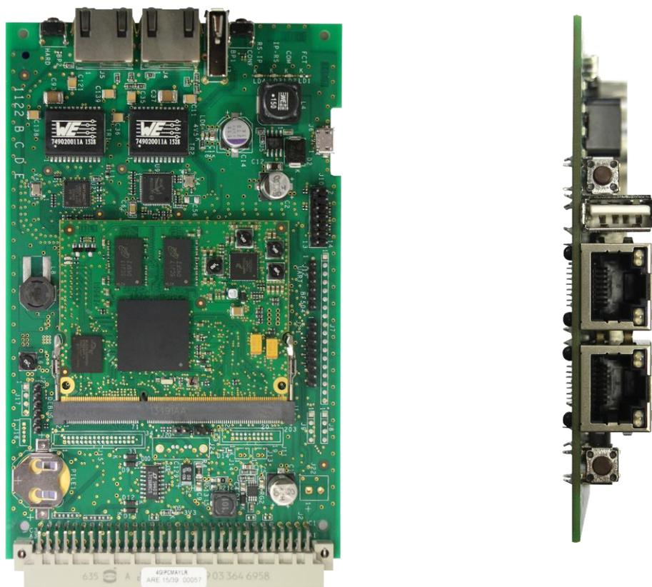
The system is connected via a 10/100 Mbits Ethernet RJ45 connection (Compatible 1Gbits) on IP1.
