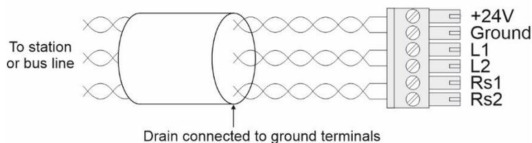
The connection between a station and the central requires a shielded twisted 3 pair cable.
