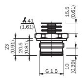
Housing with L-connector (DIN EN 175301-803 A)
