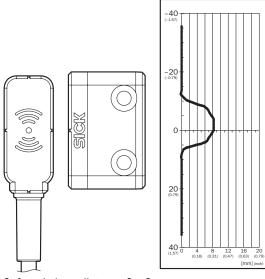
Safe switch on distance  $S_{ao}\,6~\text{mm}$
