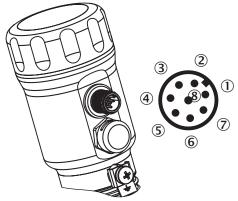
The wire colors for 8-pin cables are not uniform. Always note the pin assignment of the sensor.
