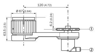
The measuring wheel circumference and surface depend on the installed measuring wheel.
